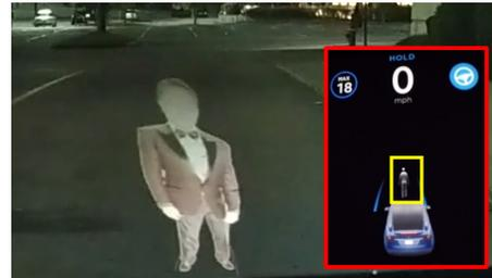
**Figure 1: In practice, despite the fact that the Tesla Model X (HW 2.5) is equipped with radar and ultrasonic sensors, it recognizes a depthless person (phantom) projected on the road in front of it as a real obstacle due to its safety policy.**
