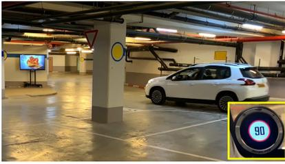
**Figure 5: Mobileye issues an alert about a phantom road sign after the phantom speed limit was detected in the upper left corner of the digital billboard.**
