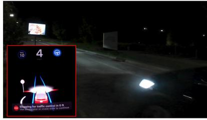
**Figure 6: Tesla’s autopilot triggers the car to stop suddenly after a phantom stop sign was detected in the upper left corner of the digital billboard.**
