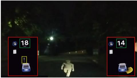
**Figure 8: The Tesla automatically driving at a speed of 18 MPH detects a phantom pedestrian that is projected on the road as a real obstacle (see a snapshot of its dashboard in the box on the left) and automatically triggers the brakes (see a later snapshot of its dashboard in the box on the right).**
