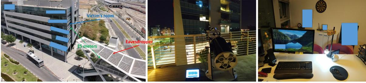
Figure 16: Experimental setup: From left to right (1) The distance between the eavesdropper (located on a pedestrian bridge) to the LED bulb of a desk lamp (in an office on the third floor of a building covered by curtain walls) is 25 meters, (2) the location of the eavesdropper, and (3) the office with the desk lamp with an LED bulb.
