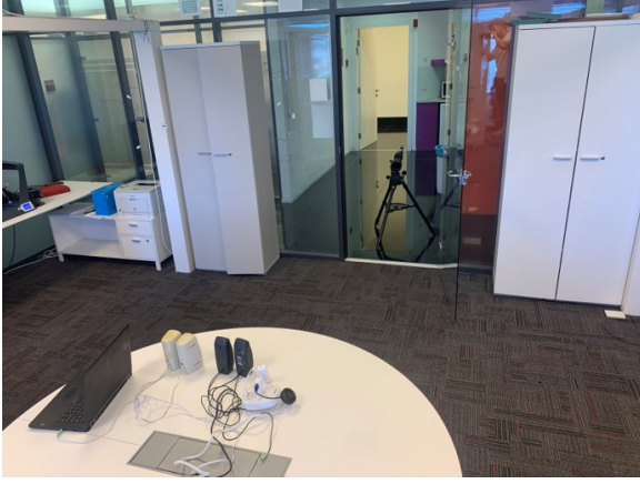
Figure 9: Experimental setup: the telescope and the four devices used in the experiments. A PDA100A2 electro-optical sensor is mounted on the telescope. The electro-optical sensor outputs voltage which is sampled via an ADC (NI-9234) and processed in LabVIEW.
